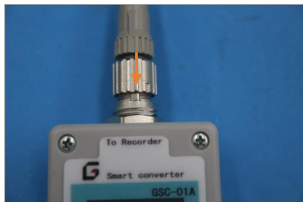
[出力側：弛み有り]
